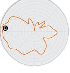
Figure 3. R560 5GHz Azimuth Antenna Pattern
