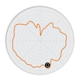
Figure 6. R560 5GHz Elevation Antenna Pattern
