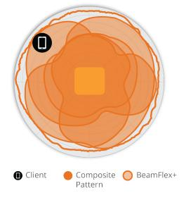
Figure 2. R560 2.4GHz Azimuth Antenna Pattern
