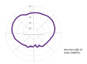
4x4 5 GHz Azimuth
