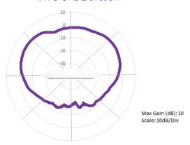
8x8 5 GHz Azimuth
