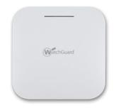
WatchGuard's AP130 access point adopts the latest generation of Wi-Fi 6 and rich WPA3 encryption, which is ideal to support low-density minimal indoor environments like a small office or remote work environments.
