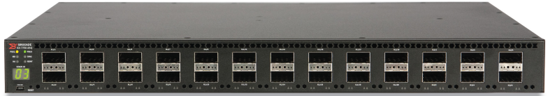
Figure 3. The Brocade ICX 7750-26Q features 26 40 GbE QSFP+ ports that can be split into as many as 96 10 GbE SFP+ ports.
