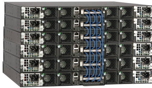
Figure 4. Up to 12 Brocade ICX 7750 Switches can be stacked using up to 12 standard full-duplex 40 Gbps QSFP+ ports per switch, providing up to 5.76 Tbps of aggregated stacking bandwidth.
