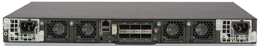
Figure 5. The Brocade ICX 7750 features hot-swappable redundant power supplies (1+1) and fans (3+1), and an optional 6 40 GbE ports module that can be used for stacking or as additional 40 GbE data ports.
